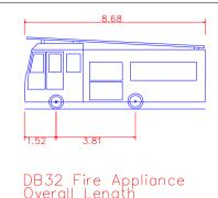
DB32 Fire Appliance Overall Length Overall Width Overall Body Height Min Body Ground Clearance Max Track Width Lock—to—lock time Curb to Curb Turning Radius
