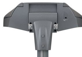
LUMA GEN2 LARGE - LED module 14000 lm - LED - Power supply unit with DALI and SystemReady interface and constant light output (integrated) - Distribution medium 31 - - - Glass - 65° x 23° - Internal (no external connection) - Side- entry for diameter 42 to 60 mm
