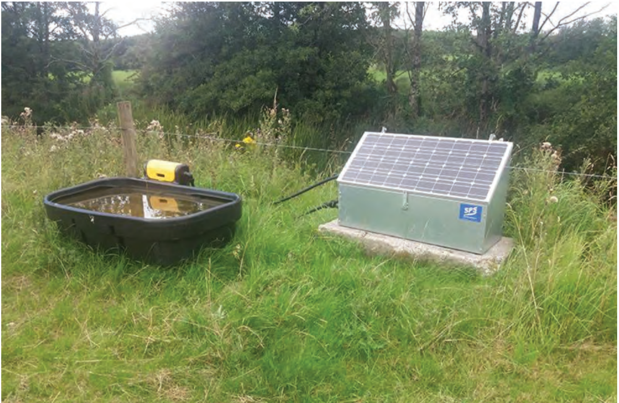
Drinking troughs to be placed at movable sites at least 20m from shore. The use of solar powered pumps allow water to be brought up the slope to troughs at various locations.
