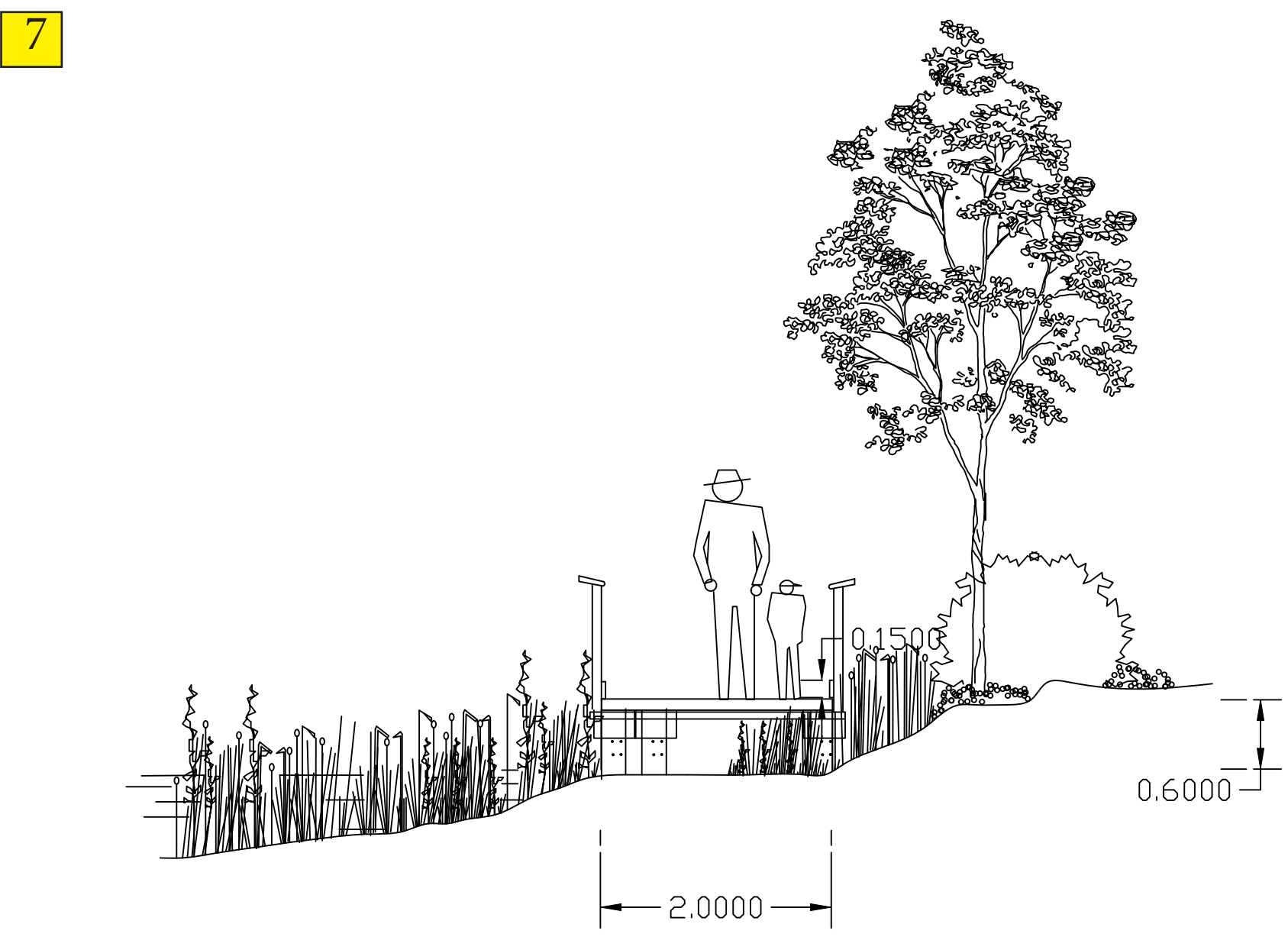
Boardwalk wide enough for wheelchairs to pass with habitat information carried on handrails. Tipping board for visually impaired and to prevent wheel escape at the board edge to be minimum 150mm high. Riparian vegetation to be allowed to renew itself beneath the board. Boards to be 600mm over water where such exists along the alignment.
